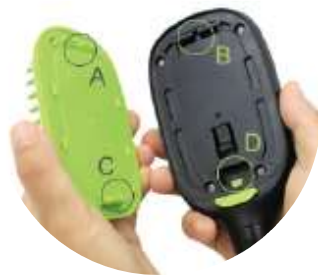
Align A with B and C with D
